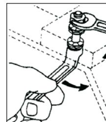
**3.** Keep the bolt/nut secured while tightening the other part (bolt/nut). For guidance on which torque to tighten with, check the Nord-Lock torque guidelines.
