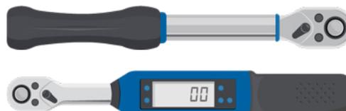
**2.** Tighten the bolt at a torque according to the Nord-Lock torque guidelines, using a calibrated torque wrench.
