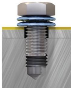
**1.** Put on the pre-assembled washer pair on the bolt and install the bolt in the threaded hole. The NLX washer shall be placed with the laser marking facing the nut or the bolts head.
