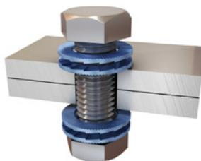
**1.** Place one pair of Nord-Lock washers underneath the head of the bolt and mount it in the through hole. Place the second pair of washers on the bolt and mount the nut.
