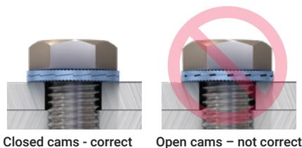
**2.** Turn both fasteners (bolt head/nut) in order to close the cams on both washers before tightening to minimize settlements.
