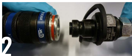
Insert the nipple into the coupling whilst the shroud is in the retract position
