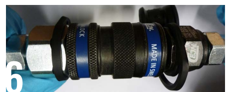
This image shows the SLS in the locked position – this joint is now safe to use
