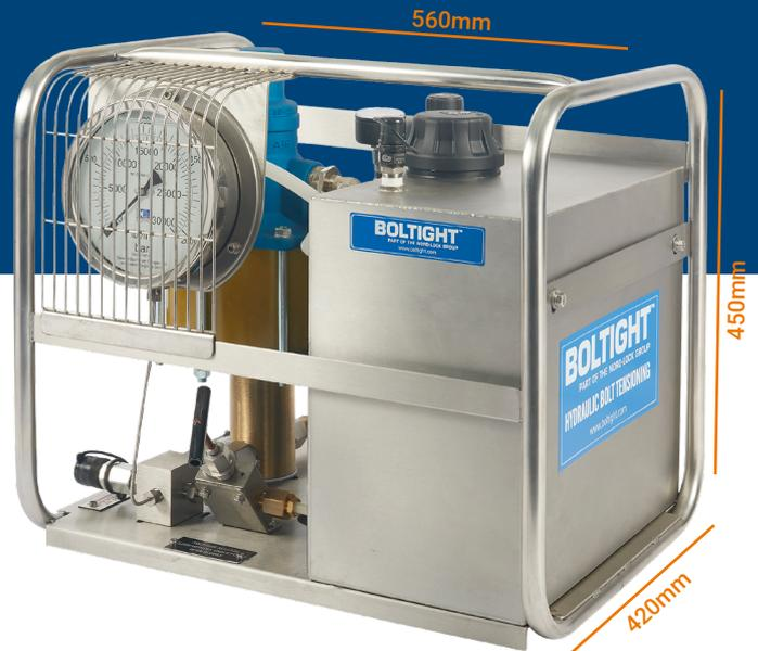
Boltight's higher oil flow, stainless steel air driven hydraulic pump has been designed for use in a corrosive environment such as Subsea. The pump has a large 15 litre oil reservoir and can be used with all Boltight 1500 bar tooling. It is ideal for projects where speed of operation is essential.
