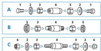
1 Bolt. 2 Washer. 3 Sleeve. 4 Axle (Pin). 5 Spanner nut. 6 Nut.
