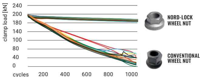
In tests, the Nord-Lock wheel nuts prove superior in securing wheel joints and maintaining clamp load. The graphs display products tightened to 200 kN and the change in clamp load during 1000 load cycles.
