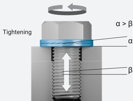
When the bolt and/or nut is tightened, the serrations grip and seat the mating surfaces. The Nord-Lock wedge-locking washer is locked in place, allowing movement only across the face of the cams.
