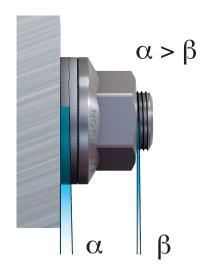
Each wheel nut is permanently attached to a pair of Nord-Lock washers. The washers have cam faces on one side and serrations on the other. When the wheel nut is tightened, the serrations on the lower washer are embedded into the mating surface.
