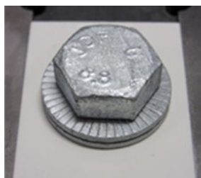
Figure 1. Tightened Nord-Lock Washer on painted surface
