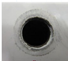
Figure 3. Painted surface after Junker Vibration test with flat washers. Random wear on the painted surface.
