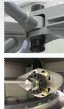
Nord-Lock Group provided Superbolt tensioners, Superbolt Expansion bolts and Nord-Lock washers for the human training centrifuge.
