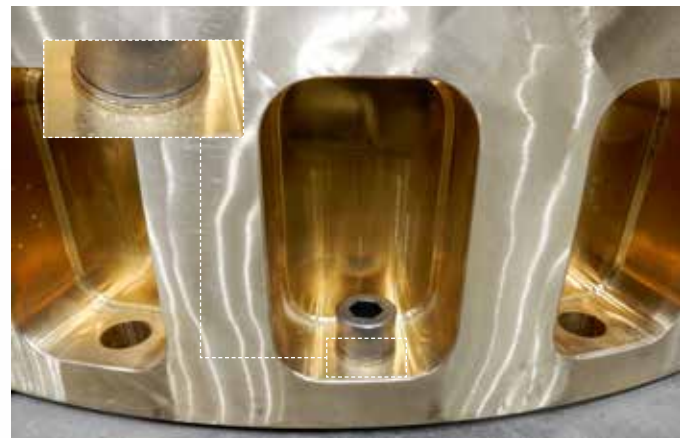
Using wedge-locking washers, it is possible to assemble propeller caps under water, saving significant amounts of money.
