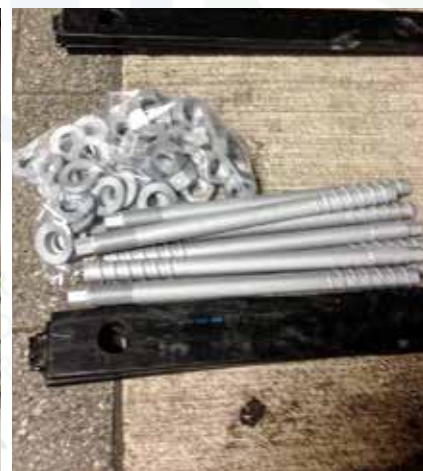
The rails of the Nuremberg underground are fitted onto longitudinal beams made of reinforced concrete using a rail mounting system, which is, in turn, connected to the tunnel floor. In recent years, the concrete stringers have been repeatedly damaged. The new concrete bolts are fitted with a patented special thread that cuts into the borehole wall upon application.
